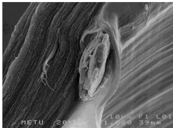
Figure 16 An SEM fractograph of VAc grafted 2°-PTFE powder filled LDPE.
