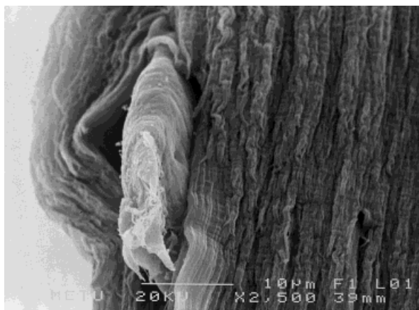
Figure 15 An SEM fractograph of St grafted 2°-PTFE powder filled LDPE.
